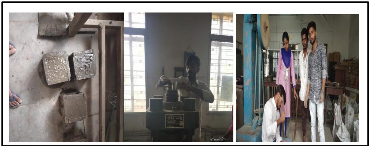
Fig II- Casting of Cubes in Lab
